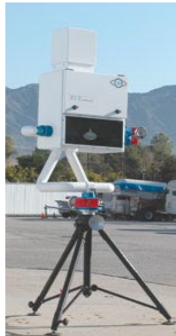
Figure 5. Driven by the limited amount of data that can be extracted using this method, Specialised Imaging in 2006 introduced a Trajectory Tracker system that allows a high-speed video camera to record over a large part of the flight path or any portion of the flight path that is of interest.
